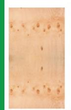
Grade according to common use for construction, Packaging, with some open and tight knots.
