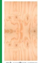
grade according to common use for construction with sanded faces and without some open, tight knots and some small open defects synthetically repaired, and / or with wood in its faces. Grade Underlayment T&G
